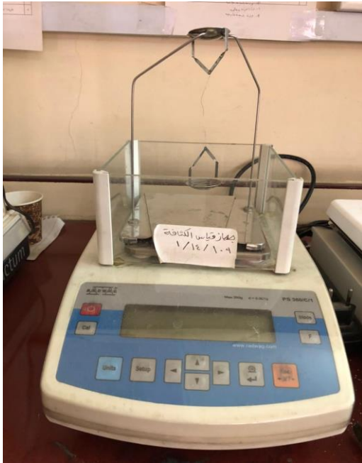
Fig. 4 the density tester.
